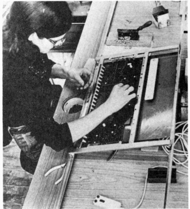
*The slide projector is synchronised with a system of small component trays which run below the assembly desk.*
