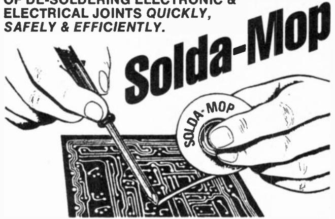
Simply place Solda-Mop on connection, apply soldering iron for about one second then remove Iron and Solda-Mop together. Two sizes:—Heavy gauge for 40/50 watt or light gauge for 10/20 watt Soldering Irons.
